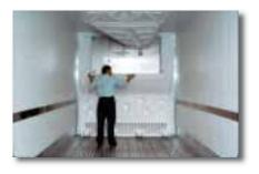
But that's just one of several benefits. This bulkhead's support pods have been uniquely designed and positioned so that return air actually mixes to deliver a more consistent temperature upon entering the evaporator coil. That results in a more efficient
