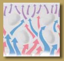
The bulkhead's support pods have been uniquely designed and positioned so that return air actually mixes to deliver a more consistent temperature upon entering the evaporator coil.
