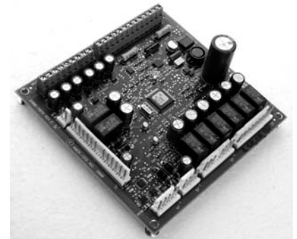
Figure 4 - RTRM (ReliaTel™ Refrigeration Module)
