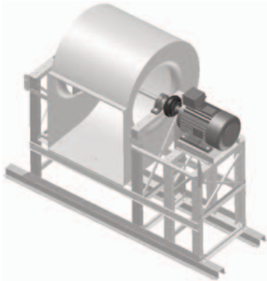
Figure 5 - Variable speed direct drive supply fan
