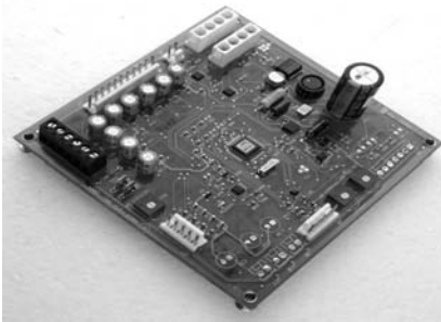
Figure 5 - RTOM (ReliaTel™ Option Module)
